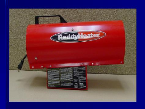
Plug the fan in first before igniting the heater. Turn the gas off before unplugging the heater. Failure to follow these steps will cause a flame that burns on the backside of the burner head, damaging the wiring and thermal switch.
