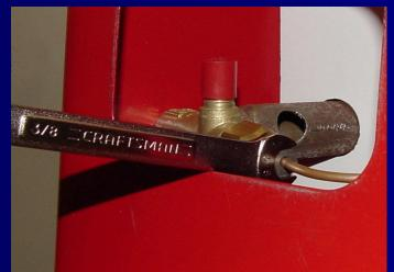
If the heater still shuts off and does not run correctly there could be a problem with the thermocouple or the valve.
